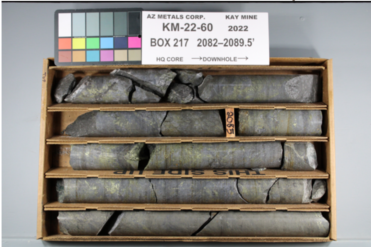
Figure 3. Hole KM-21-60 displaying interval from 634.3 m to 635.5 m downhole, intersecting 1.2 m grading 273.0 g/t Au, 5.6 % Cu, 0.2% Zn, and 715 g/t Ag. This is part of a broader 93.3 m interval, from 554.7 to 648.0 m, grading 8.3 g/t AuEq. See Table 1 for constituent elements, grades, metals prices and recovery assumptions for AuEq g/t calculations. Analyzed Metal Equivalent calculations are reported for illustrative purposes only.
