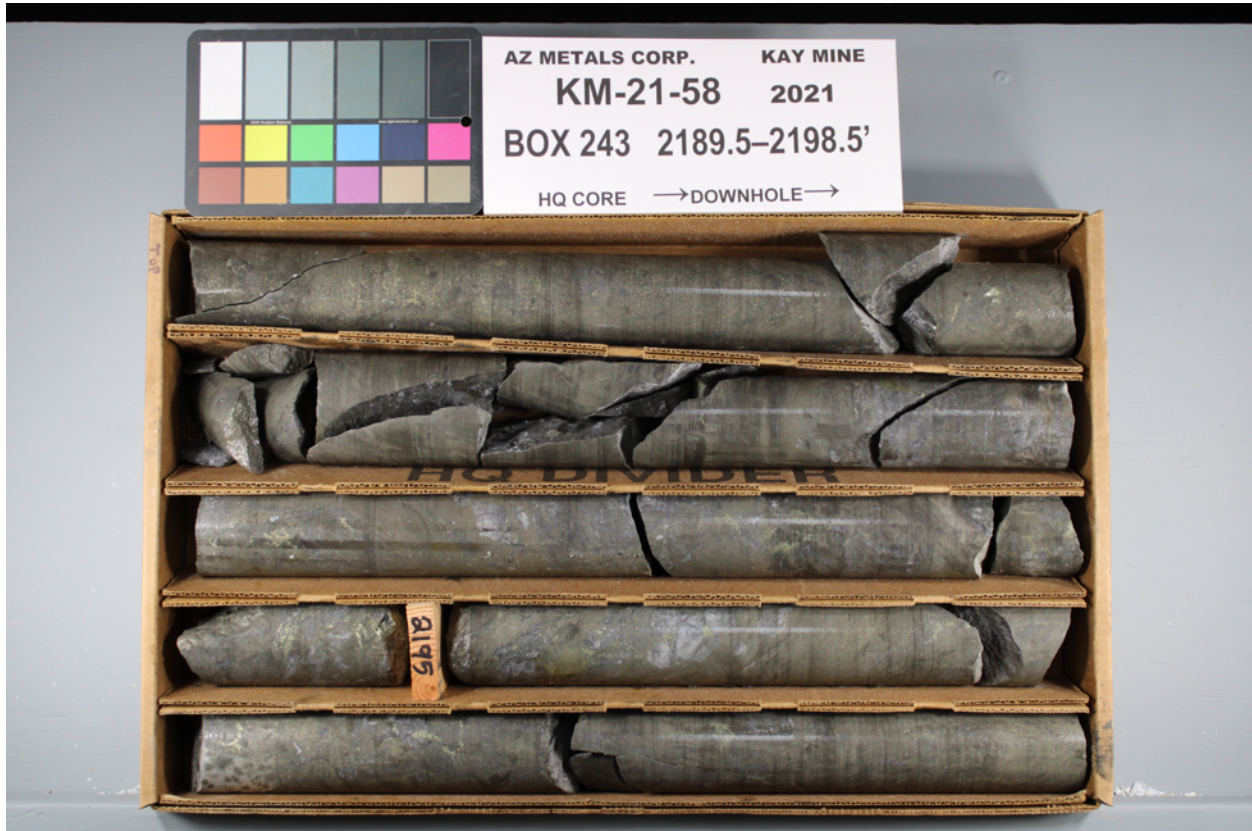
Figure 3. Hole KM-21-58 displaying interval from 667.8 m to 670.5 m downhole, intersecting 1.5 m grading 43.2 g/t Au, 2.6% Cu, 7.8% Zn, and 856 g/t Ag. This is part of a broader 68.4 m interval, from 614.2 m to 682.6 m, grading 6.7 g/t AuEq. See Table 1 for constituent elements, grades, metals prices and recovery assumptions for AuEq g/t calculations. Analyzed Metal Equivalent calculations are reported for illustrative purposes only.
