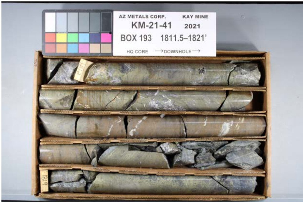
Figure 5. Hole KM-21-41 displaying interval from 552.5 m to 555.4 m downhole, part of a broader interval (from 546.7 m to 558.1 m) of 11.4 m grading 5.9% Cu, 5.8 g/t Au, 3.2% Zn and 185 g/t Ag.
