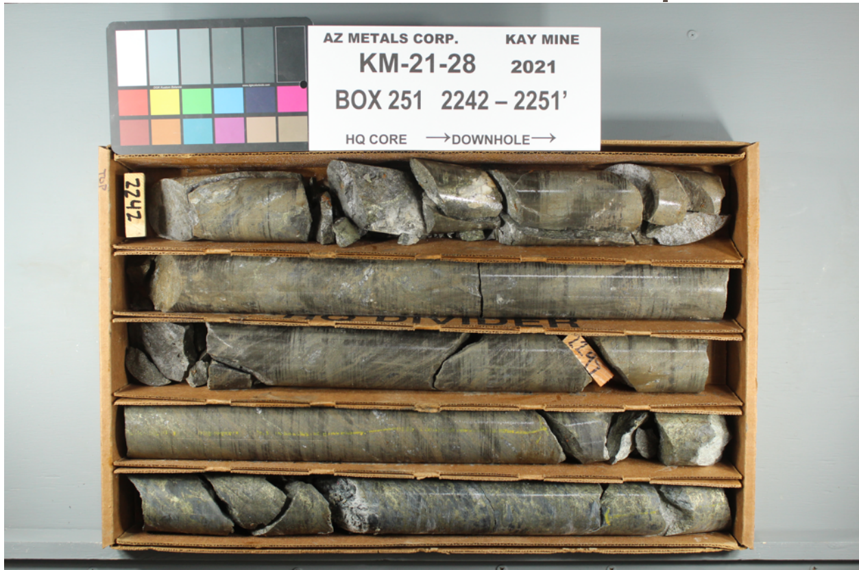
Figure 4. Hole KM-21-28 displaying interval from 681.8 m to 684 m downhole, part of a broader interval (from 681.1 m to 689.0 m) of 7.9 m grading 4.4% Cu, 9.5 g/t Au, 10.3% Zn and 93 g/t Ag.
