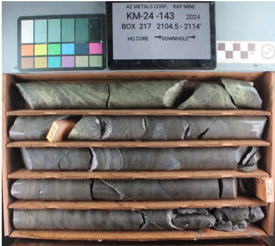
Figure 3. Drill core from Hole KM-24-143, showing part the 3.2 m interval 640.8 m to 644 m which intersected 4.1 g/t gold, 8.2% copper, 8.6% zinc, and 291 g/t silver (for an equivalent grade after assumed recoveries of 14.9% CuEq). This is part of a broader interval of 20.1 m grading 3.4% CuEq.
