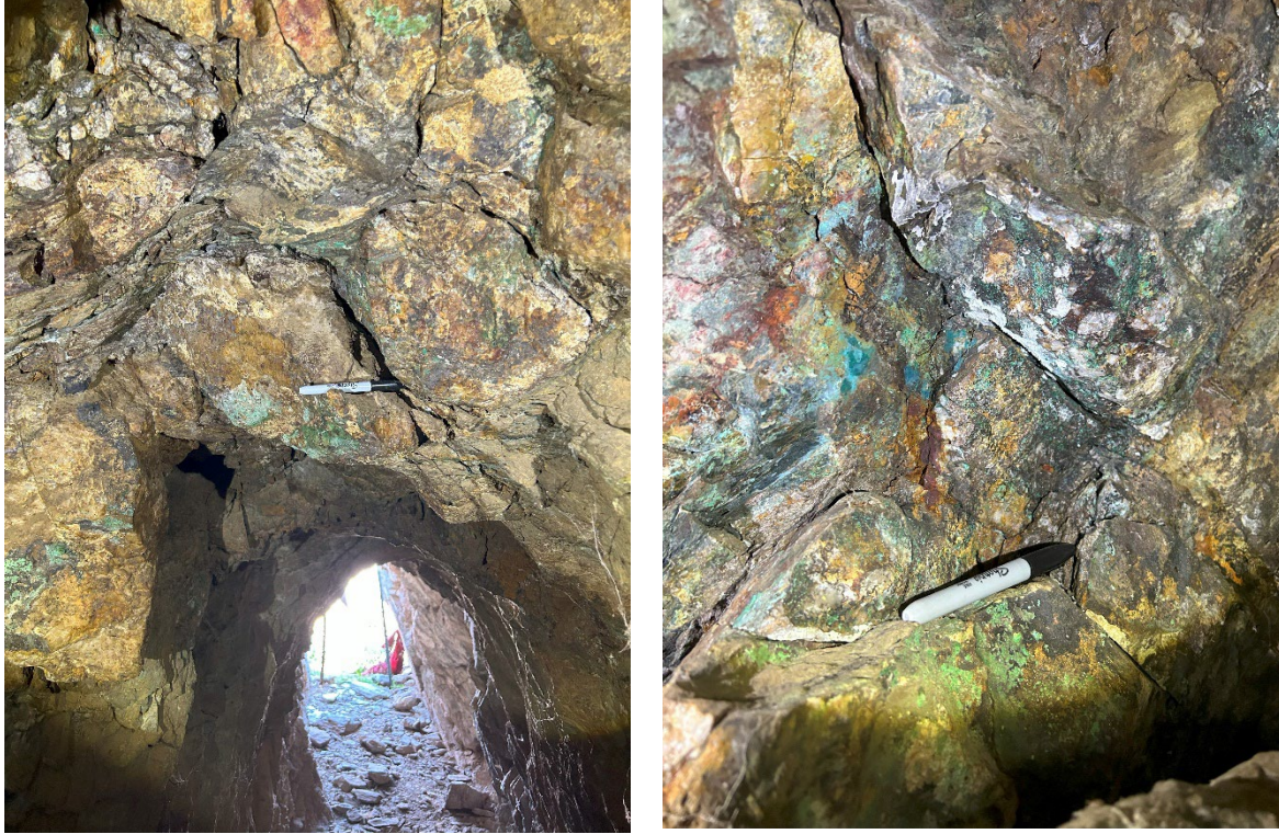
Figure 2. Left: historic adit on newly-staked northern claims showing copper staining. Right: sulphide mineralization with copper oxide staining. Sampling returned grades of 11.7% Cu, 6.7 g/t Au, 9.1% Cu, and 286 g/t Ag.
